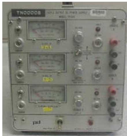
Scientific lab desktop power supply with three separate voltage supplies.
